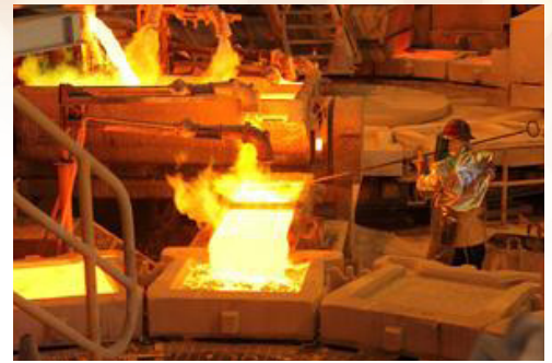
Blister copper from the smelter is poured into the anode casting moulds. The anodes are cast into slabs about 1 metre square with arms at the top corners for lifting. (Courtesy of Codelco.)
