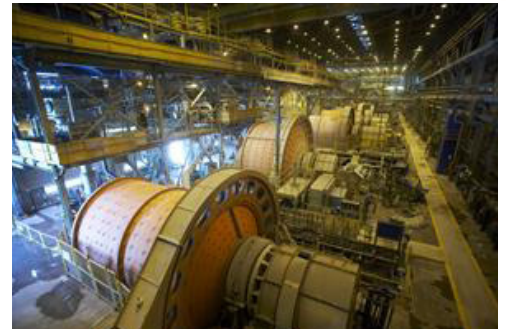
Ball mills crush the ore into a fine powder. (Courtesy of Rio Tinto.)
