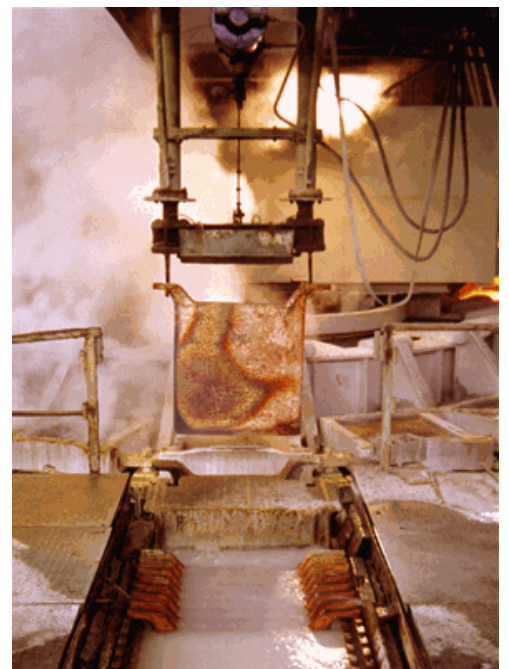
Lifting the solidified anodes into cooling tanks. (Courtesy of Codelco.)
