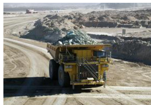
This truck carrying copper ore has no driver. It is guided by a GPS system. Can you see the GPS antenna? (Courtesy of Codelco.)
