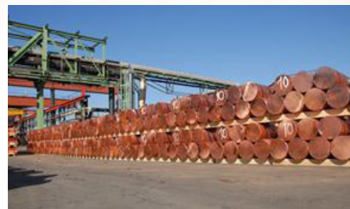
Cathode copper is remelted and cast into billets ready for turning into copper products. (Courtesy of Aurubis.)
