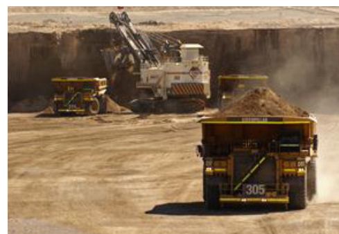
Copper ore is loaded into trucks. In some mines these trucks have no driver. (Courtesy of Codelco.)
