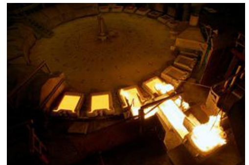
The anode casting turntable moves slowly round. The anodes can be lifted out at the far side. (Courtesy of Codelco.)
