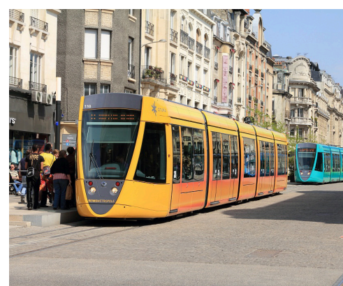
This tram line in Reims uses a central power track in the ground to avoid spoiling the city with overhead lines. Power is supplied to the track by copper cables. The track is only live beneath the tram. The tram is driven by copper wound induction motors. (Wikimedia Commons.)
