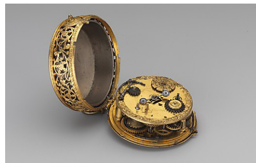
This gilded brass watch was made in London and dated 1600-1610. Brass is non-magnetic and easy to machine into fine gears. (Courtesy of Metropolitan Museum of Art.)
