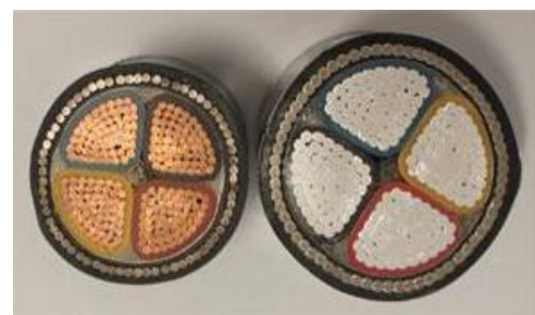
Cables made from copper and aluminium. The aluminium cable has nearly twice the area to give it the same resistance as the copper cable. You can see the strands of conductor and the armour.
