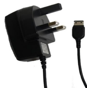
Mobile phone chargers contain a step-down transformer to convert the input of 220 V to a working output voltage of around 5 V.
