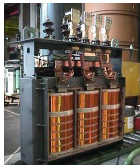
Copper windings in a transformer.
