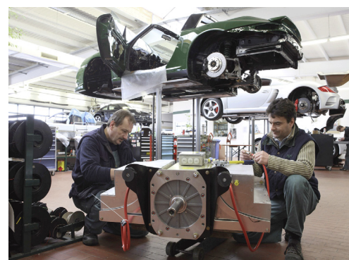
Figure 11: An electric motor and batteries replacing a petrol engine in a Porsche car. (Courtesy of Siemens.)
