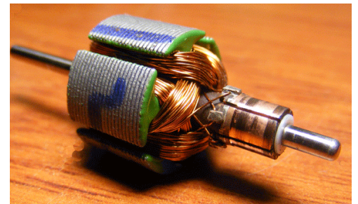
Figure 8: A DC motor rotor with coils and commutator. More coils and segments give a more continuous turning force. (Wikimedia.)
