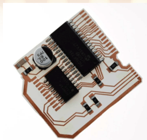
Printing of copper circuit tracks directly onto thin flexible plastic is making small, lightweight and very low cost electronics possible. Copper is only deposited on the tracks. This minimises waste. (Courtesy of Conductiveinkject.)
