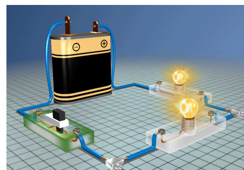
Figure 1 - The current is the same everywhere in this circuit, but the copper stays cool while the lamps get hot. Electrons have a hard time getting through the lamps and lose a lot of energy in collisions. This is converted to heat. They have an easy ride through copper, losing almost no energy at all. (Courtesy of Gida.)
