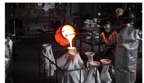
Bronze is melted in a crucible. Bronze melts at about 1000 °C. It is heated to a higher temperature of 1150 °C to pour into moulds of sand or ceramic. The higher pour temperature prevents premature solidification in narrow parts of the mould and reduces the viscosity of the molten bronze. (Courtesy of artworksfoundry.com.)
