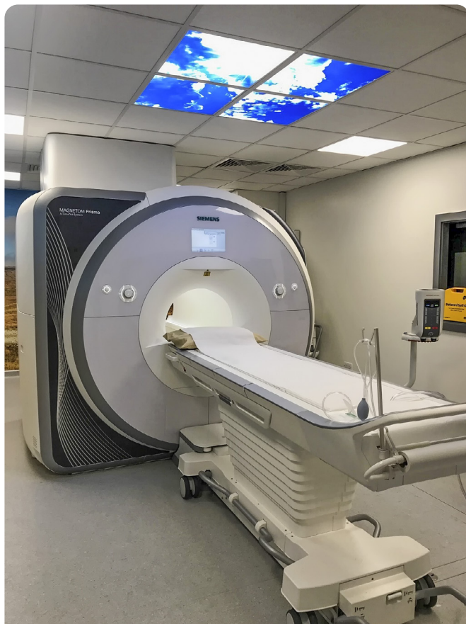
Figure 6 The MRI scanner in which I twice spent a 'relaxing' hour or so, lying on the area covered with the white sheet. The top part of the trolley could slide through the hole in the centre, taking me with it and stopping to scan the regions required. The bright blue-and-white sky above is not real, the clouds never move. The room is on the ground floor of a high building and has a false ceiling, it is probably provided as a calming influence for apprehensive patients.
