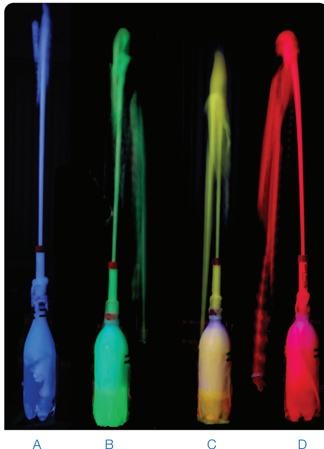
Figure 3 The Mentos eruption in the presence of fluorescent dyes and illuminated with 365 nm UV light. In each case, two Mentos were added via a geyser tube. A: tonic water; B: lemonade + Tesco Lemon All Purpose Cleaner (40 cm 3 cleaner added to 1 dm 3 of lemonade); C: lemonade + rhodamine 6G ( 1.5 \times 10^{-5} mol dm -3 ); D: lemonade + rhodamine B ( 1.5 \times 10^{-5} mol dm -3 ).
