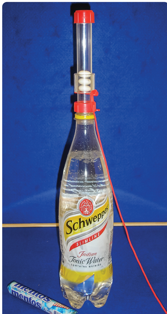
Figure 1 Geyser tube arrangement with three Mentos in place; removal of the pin (located just underneath the Mentos) releases the Mentos into the bottle
