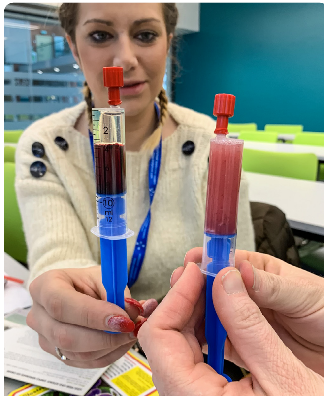
Figure 5 Syringes with caps can be used to demonstrate immiscible liquids and then the effect of adding an emulsifier
