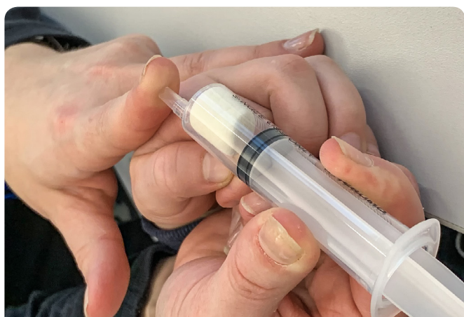
Figure 2 The pressure change in the syringe can cause a foam such as a marshmallow to expand or contract
