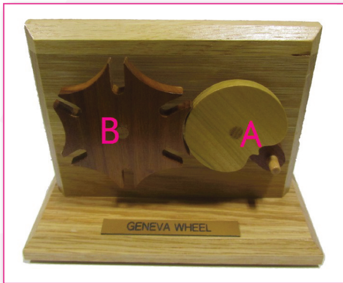
Figure 3: Geneva wheel model system.
