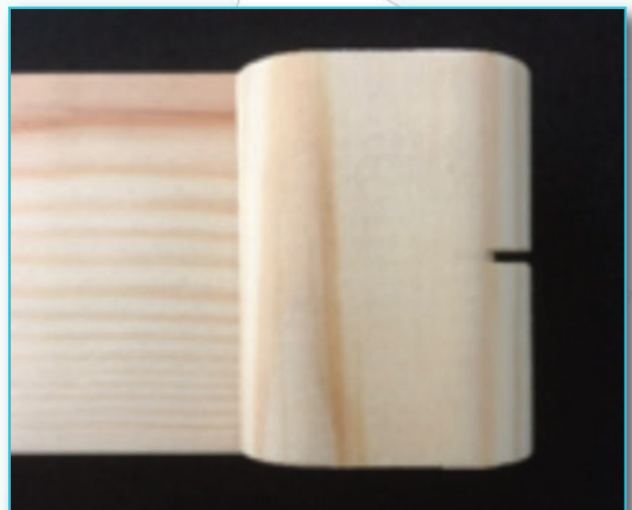
Figure 7c: A groove cut in the D-piece holds the pendulum thread.
