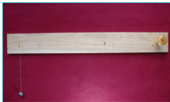
Figure 3: An historically-accurate reconstruction of Santorio's beam-type pulsilogium (Bigotti et al , 2017).
