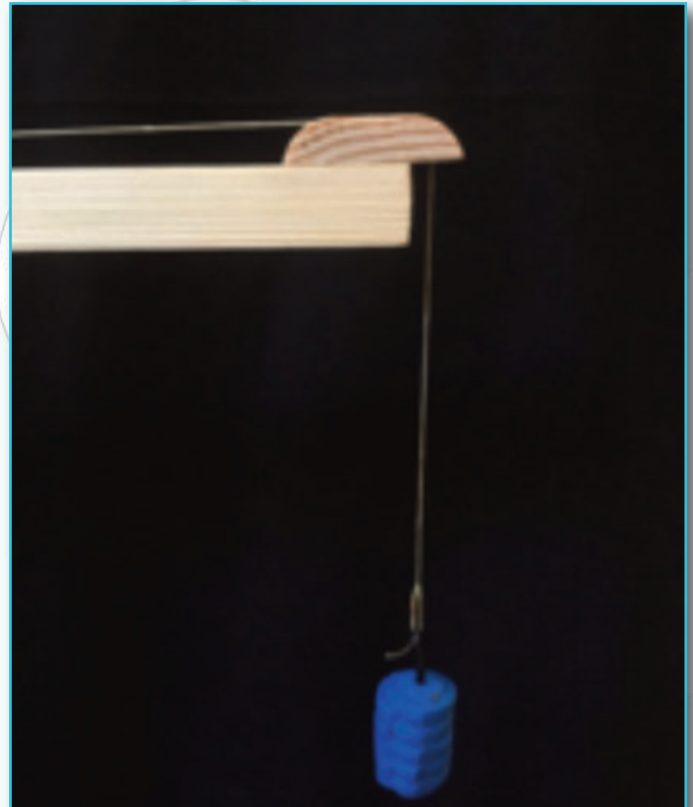
Figure 7c: A groove cut in the D-piece holds the pendulum thread.
